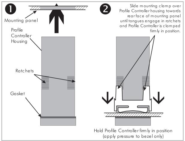
Figure 1-3 Panel-Mounting the Profile Controller
